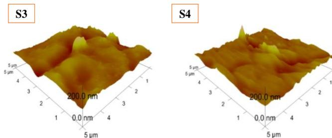
Fig. 2. 3D AFM images of the surface of the samples Sm 3, and Sm 4 with scan area  $5 \times 5 \mu\text{m}^2$  and z-range,  $z = 200 \text{ nm}$
