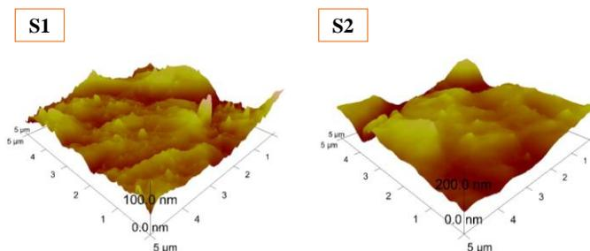
Fig. 1. 3D AFM images of the surface of the samples Sm 1, and Sm 2 with scan area  $5 \times 5 \mu\text{m}^2$  and z-range,  $z = 100 \text{ nm}$  and  $z = 200 \text{ nm}$
