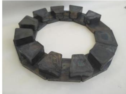
Fig. 3 The stator of a prototype two-stator electric motor using a composite soft magnetic material based on ASC100.29
