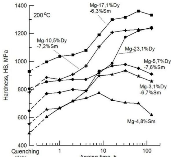
Fig.1. Hardness of the Mg-Dy-Sm alloys as a function of aging time at 200°C
