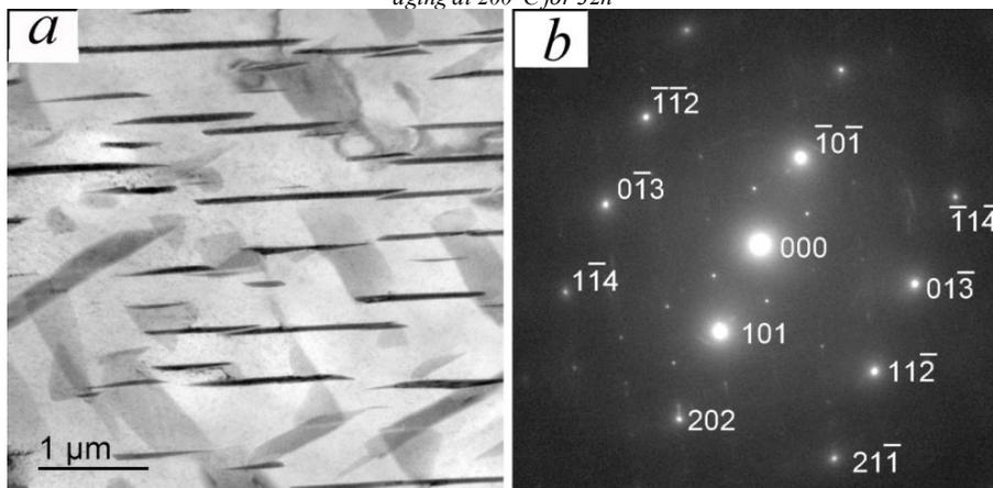
Fig.5. TEM image of the microstructure (a) and diffraction pattern, zone [-131] (b) of the Mg-5.7%Dy-7.6%Sm alloy after solution treatment and aging at 250°C for 128 h.
