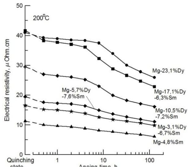
Fig.2. Electrical resistivity of the Mg-Dy-Sm alloys as a function of aging time at 200°C
