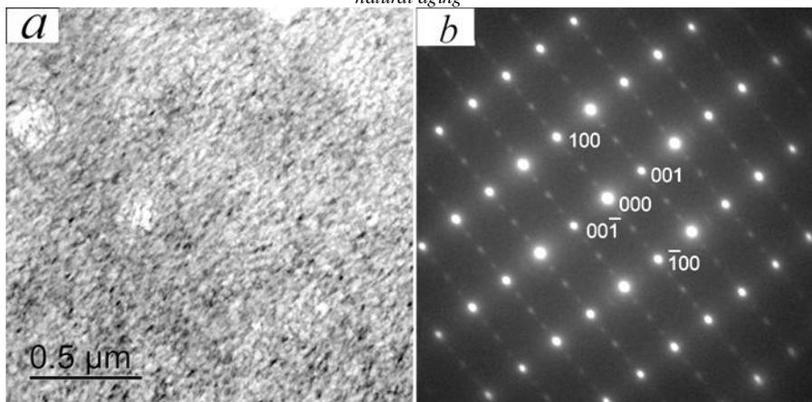
Fig. 4. TEM image of the microstructure (a) and diffraction pattern, zone [010] (b) of the Mg-5.7%Dy-7.6%Sm alloy after solution treatment and aging at 200°C for 32h
