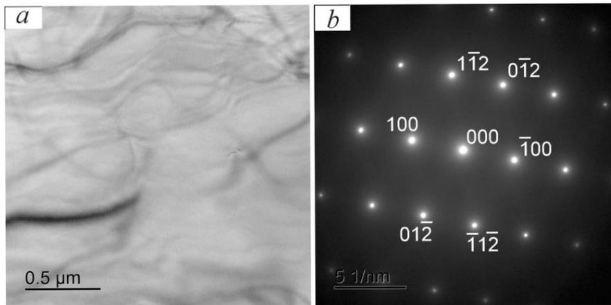
Fig.3. TEM image of the microstructure (a) and diffraction pattern, zone [011] (b) of the Mg-5.7%Dy-7.6%Sm alloy after solution treatment and natural aging
