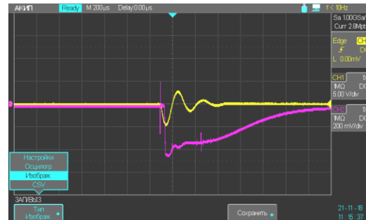
Fig. 5. Synchronous oscillograms of current pulse (CH1) and the radiation (CH2) of the contact zone of Fe-Cu metal welding (capacitive energy storage voltage U_{max} = 2.2 kV).
