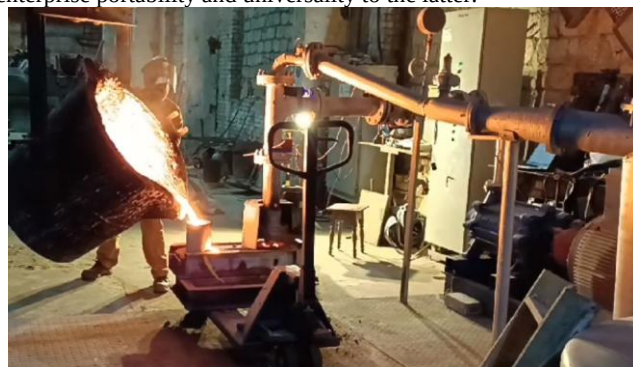
Fig. 2. Pilot installation for hydrovacuum dispersion of metallurgical melts, implemented in "Geo Enterprise" LLC
