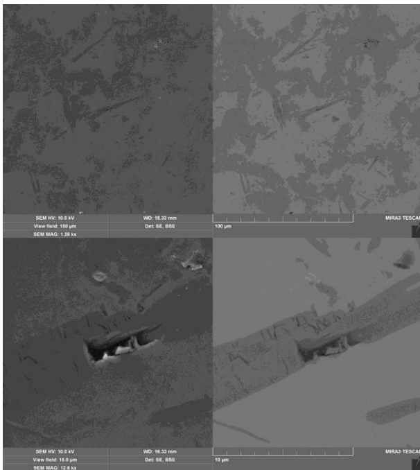
Fig.3. Hot-pressed MMC at temperature 1300 °C
