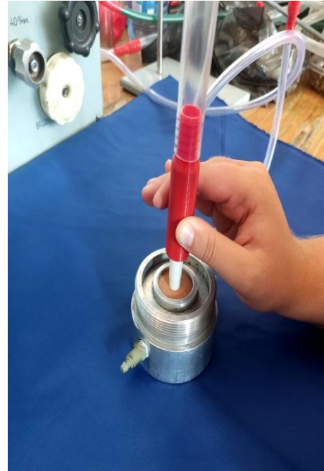
Fig. 4. Local permeability measurement process.
