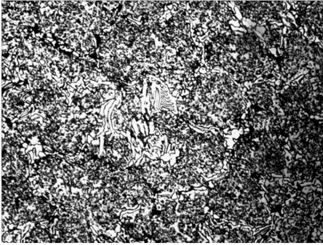
Fig. 6. Ledeburitic eutectic in steel 2 after stamping, 800x
