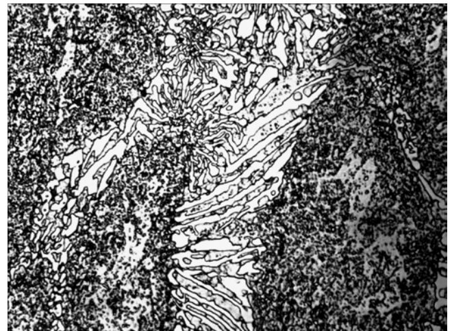
Fig. 5. Ledebouritic eutectic in steel 1 after stamping, 800x
