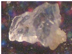
Fig.4 Geometry of a sand grain and sand with conditions of better adhesion to the binder
