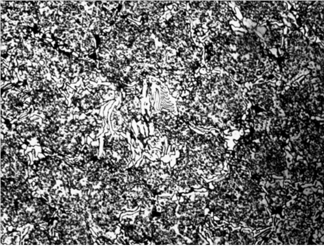
Fig. 6. Ledebouritic eutectic in steel 2 after stamping, 800x
