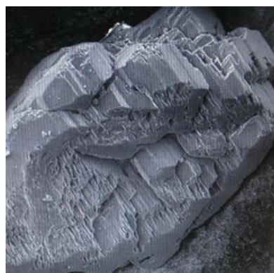
Fig.1 Defects – cracks and pores on surface of the sand grain
