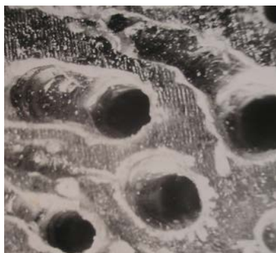
Fig. 8 Gasous pores and canals in the hardened binding composition
