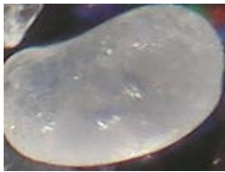
Fig.4 Geometry of a sand grain and sand with conditions of better adhesion to the binder
