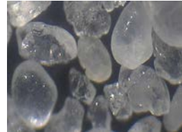
Fig.4 Geometry of a sand grain and sand with conditions of better adhesion to the binder
