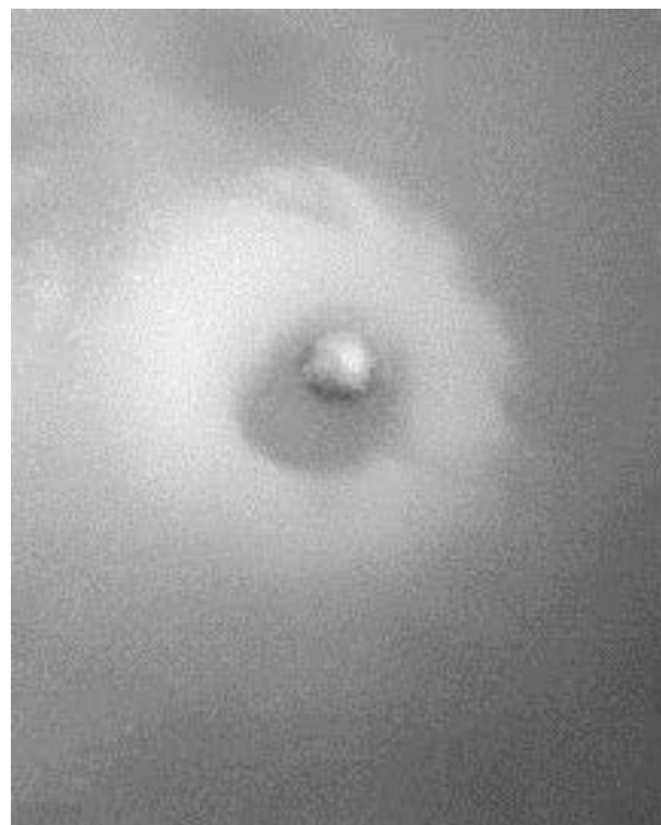
Fig. 5 Ferrogram from oil diesel engine. Spheroid always indicates the development of fatigue crack. Magnified 1000 x.
