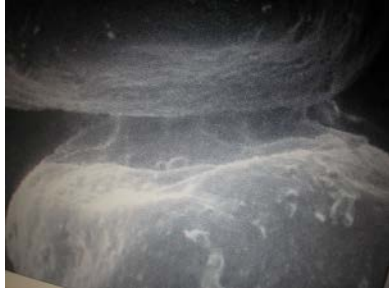
Fig. 3. "Linking bridge" between two sand grains
