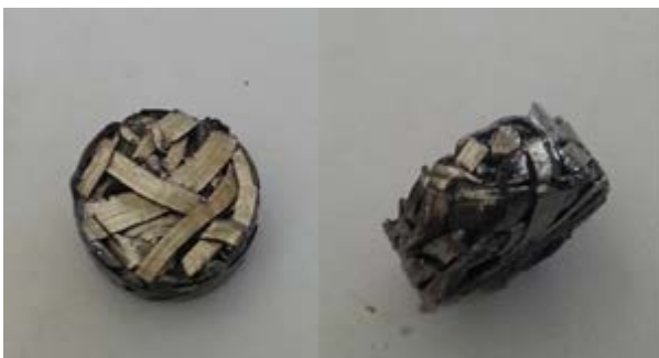
Fig 1. Photographs of H13 tool steel preforms
