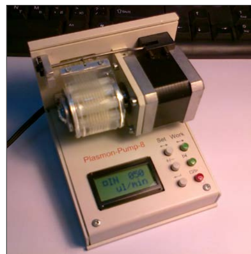
Fig.3. Appearance of the peristaltic micro-pump
