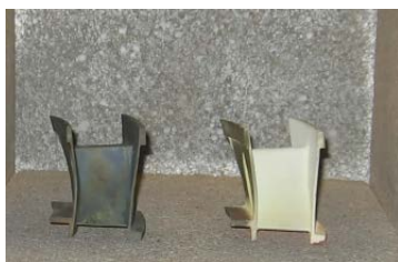
Fig. 1 The turbine blades: left – without TBC, right – with TBC.
