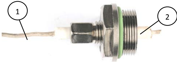
Figure 3: Silver-silver chloride sensor optimized for the corrosion chamber
