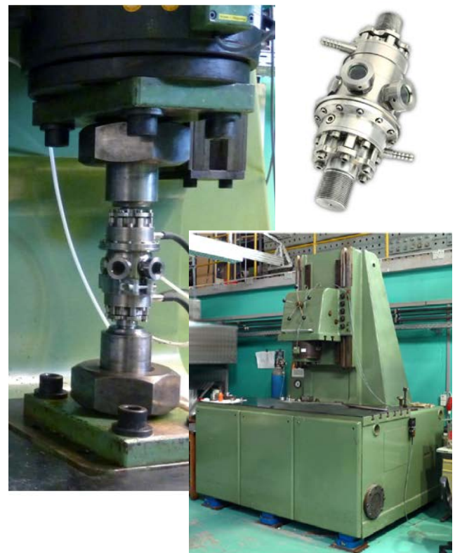
Figure 2: Experimental set-up: corrosion chamber applied to resonance testing machine
