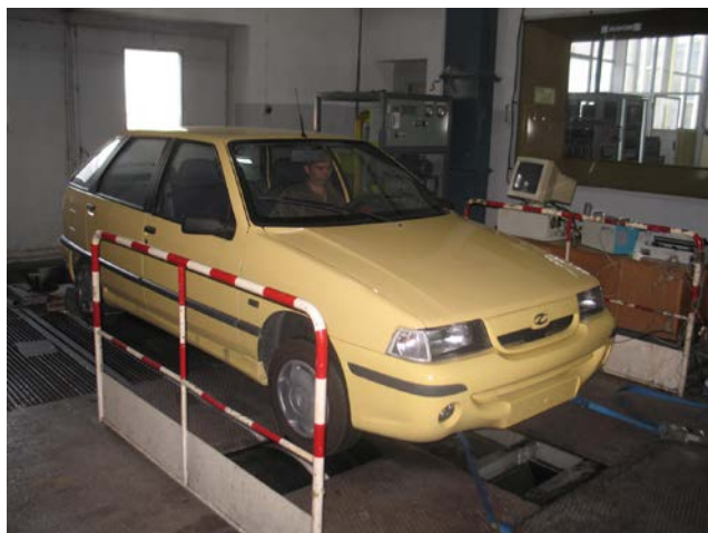
Fig. 2 Investigations of vehicles on rolls
