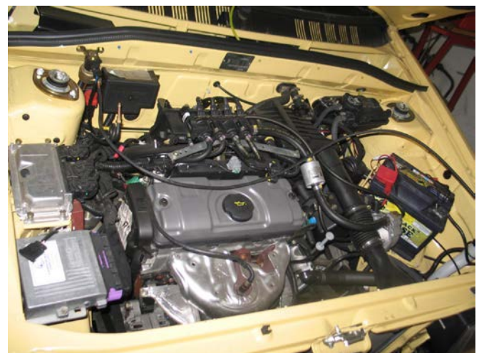
Fig. 1 Vehicle Florida 1.6 In L- OMEGAS Landi Renzo
