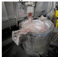
Figure 9 Pouring of molten metal from the melting furnace, LTH Learnica
