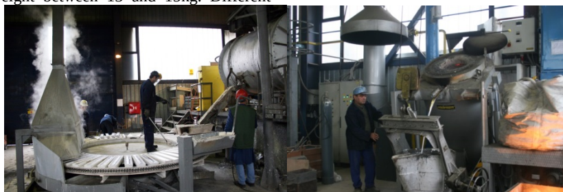
Figure 5 Agregates for melting aluminium alloys ina RZ Institut
