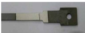
Fig. 6. Delamination of top alumina plasma-sprayed coating after testing of tensile specimen (a photo of specimen – a, schematic sketch – b)
