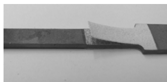
Fig. 5. Schematic sketch of the dog-bone-shaped specimen with top coat/bond coat system before testing
