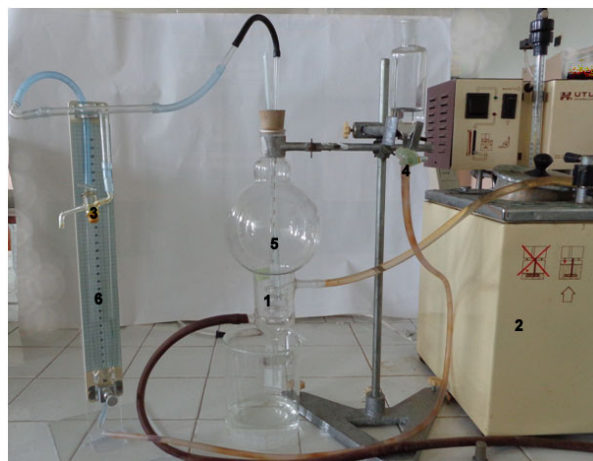
Fig. 1 Laboratory apparatus for measuring a surface tension.
