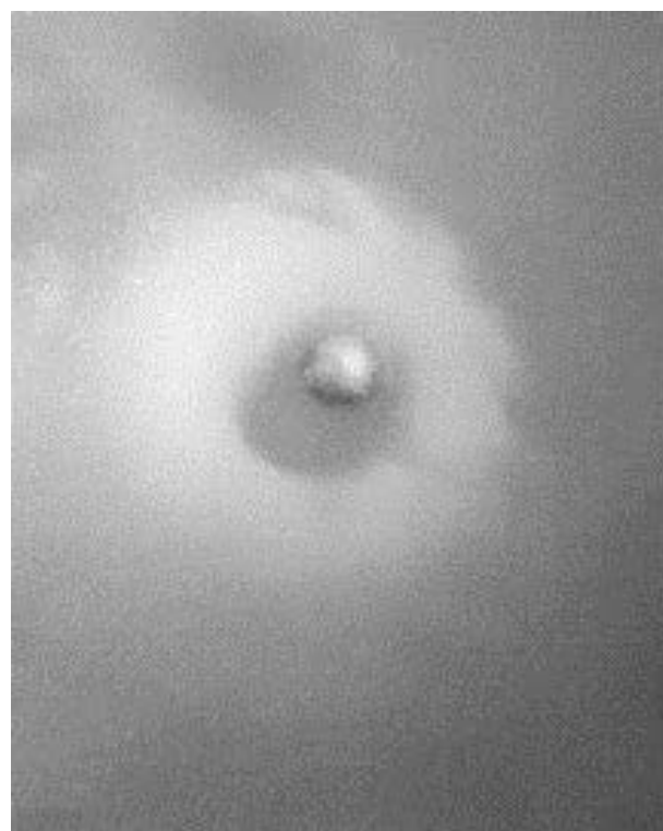
Fig. 5 Ferrogram from oil diesel engine. Spheroid always indicates the development of fatigue crack. Magnified 1000 x.
