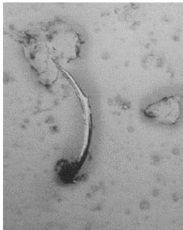
Fig. 4 Strong cutting wear steel particle, so-called two-point abrasion. Harder member of the friction pair penetrates into softer member of friction pair and separates chips from it. Magnified 1000 x.
