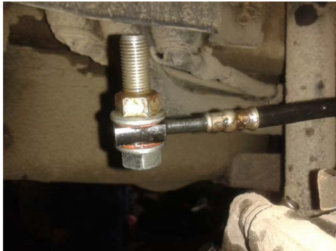
Fig. 3 Seal at the end of the brake pipe. The rear axle of the vehicle - Skoda Octavia. Source: Authors
