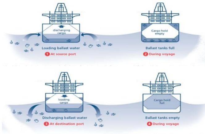
**Figure 2.** Ballast exchange between ports (IMO GloBallast)
