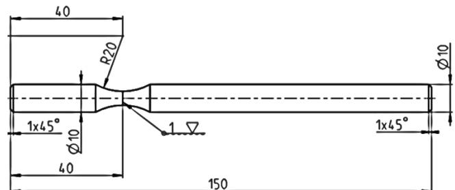
Fig. 2: The geometry of the testing sample for the fatigue testing status
