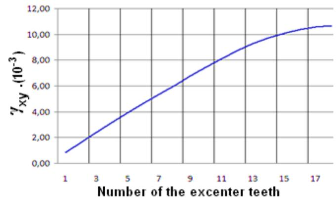
Fig. 7: Values of the strain at the torsion stress of the welded samples,  $e = 4$  mm, material AlMgSi07
