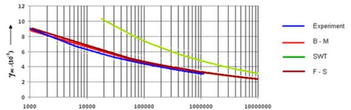
Fig. 10: Comparison of Manson-Coffin's curves of chosen fatigue criterions for the valuation of low cycle uniaxial fatigue and from experimentally achieved values at torsion stress of samples
