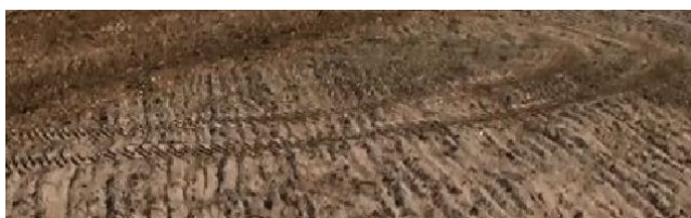
Fig. 14. No visible ground deformation during TVU turning (picture made by video camera mounted on KoBE) 1
