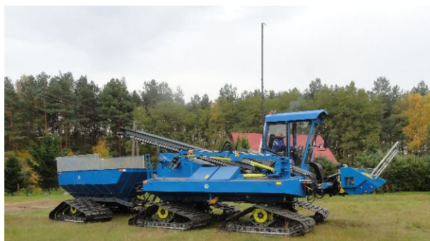
Fig. 8. TVU ready to preliminary field test, on the top of mast is mounted Racelogic's HD video camera. Presented version of tractor and trailer is an amphibian unit that should be able to move through water (lakes, channels) (October 2013) 1
