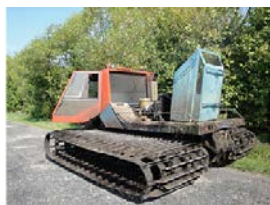
Fig. 1. Ratrac adapted by farmer to work on wetlands, blue color cover is open - for better cooling of the engine 1 □
