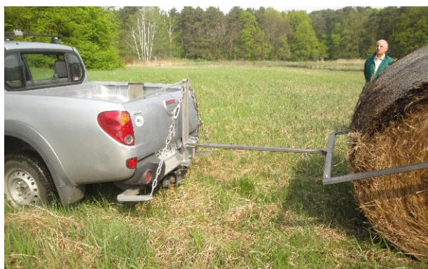
Fig. 19. Mitsubishi L200 research truck with bale (dia. 1,8 m) [9]
