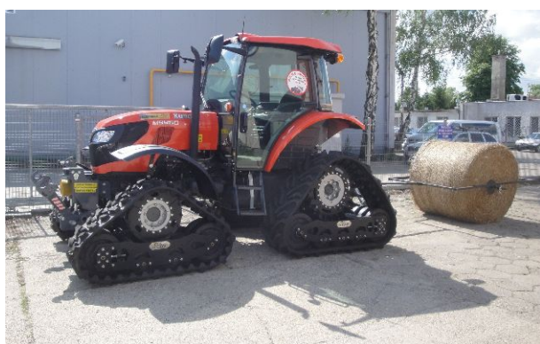
Fig. 20. Kubota M9960 tractor with delta tracks module made by Soucy Track, Canada 1 [12]
