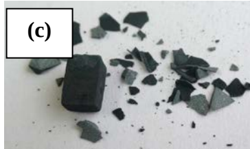
Fig. 3. Images stainless steel and joint after thermogravimetric measurement: (a) TP347HFG, (b) joint, and (c) VM12-SHC.
