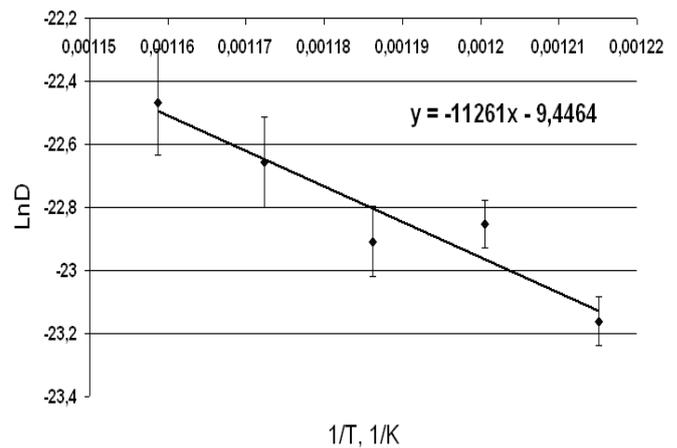
Fig3. Estimation of  $E^*$  with the help of linear temperature diffusion coefficient dependence
