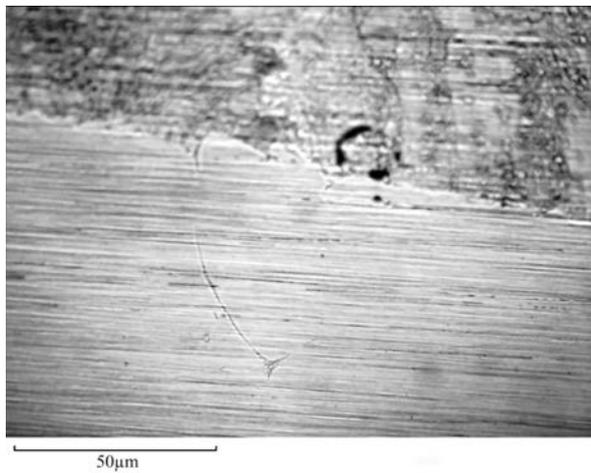
Fig. 2. Morphology of the liquid bismuth penetration
