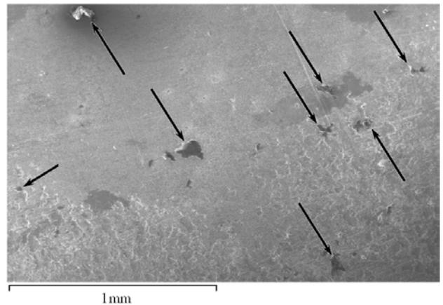
**Fig.1.** Appearance of melt on the opposite sample's surface. Arrows show the penetration points
