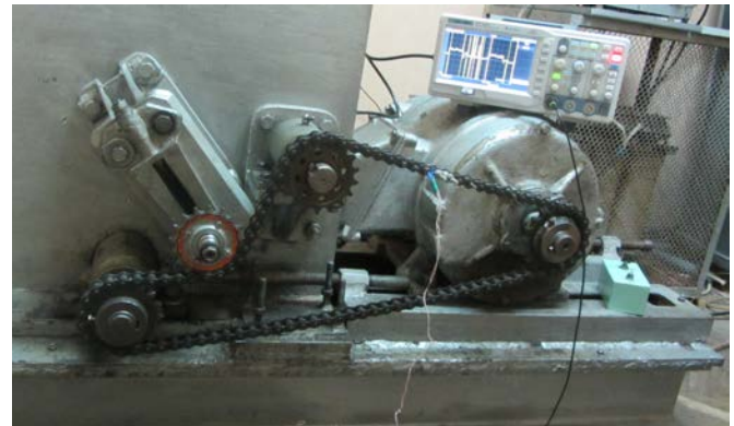
Fig. 13. The experimental stand is equipped with a metal chain transmission
