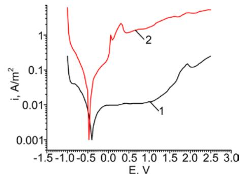
**Fig. 4** Potentiodynamic curves of Ti-6Al-4V alloy with oxynitride coatings in 0.9 % NaCl solution at 36 °C (curve 1) and 40 °C (curve 2).
