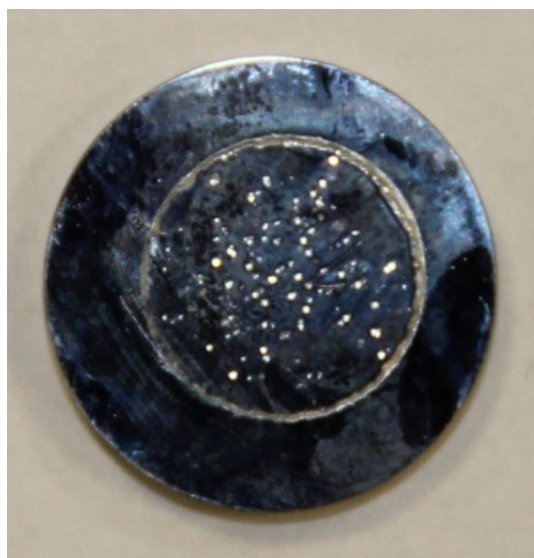
Fig. 4. Appearance of coupon made from steel 2 Cr18Ni10N (N=0.186 %) after testing in environment 3% NaCl
