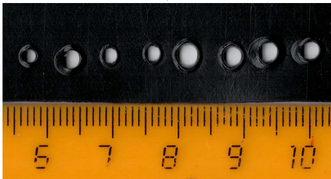
Fig. 7. Example of perforation of sheet of textolite (a) and polyethylene film (b) which is filled with soot.
