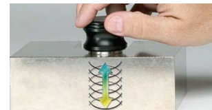
Fig.4. Transducers with X-cut of piezo-electric element
