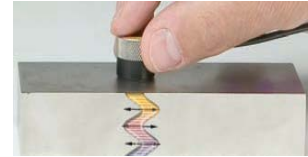
Fig.5. Transducers with Y-cut of piezo-electric element
