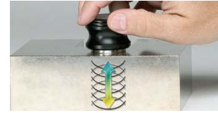
Fig.4. Transducers with X-cut of piezo-electric element
