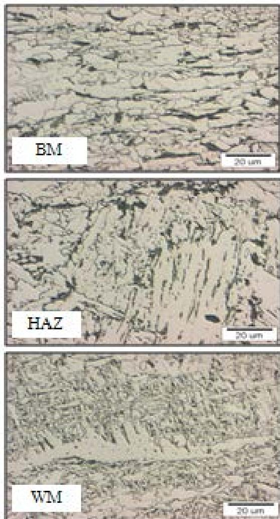
**Fig.8** Microstructure of welded joint
