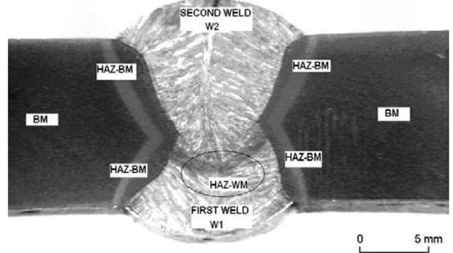
Fig.4 Schematic illustrating of metallographic specimens
