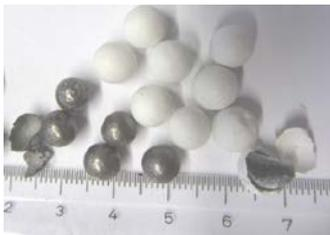
Fig. 2 Iron hollow balls (kaolin coated and non-coated)
