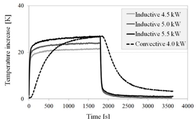
Fig. 3 Influence of the energy input on the heating behavior
