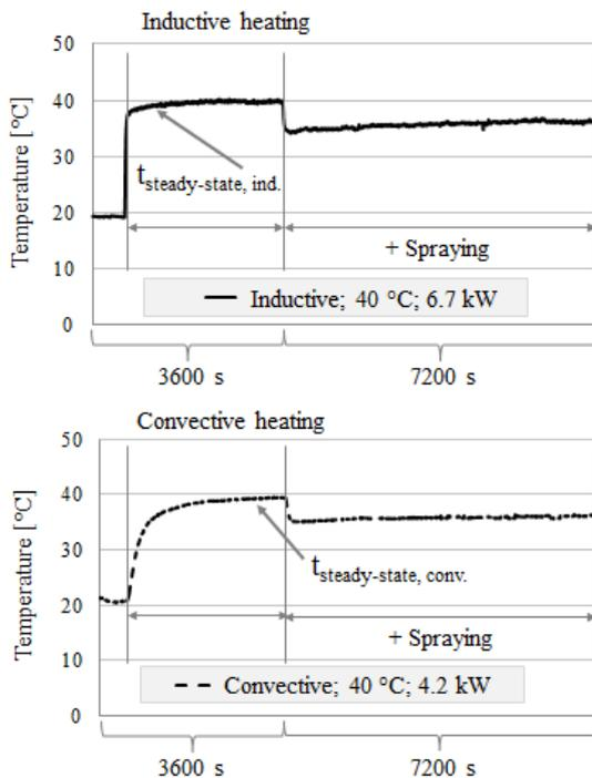
Fig. 5 Temperature profile of suspension drying process
