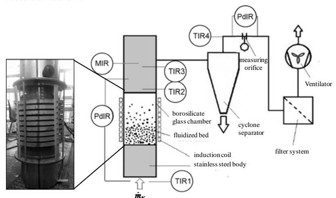
**Fig. 1** Schematic design and picture of the inductive experimental plants
