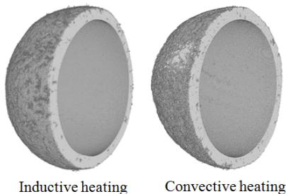
**Fig. 11** 3D reconstruction of granule shells using micro-computed X-ray tomography
