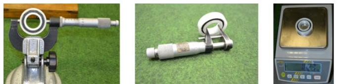
Figure 5: Measuring instruments used in the measurement of geometry change
