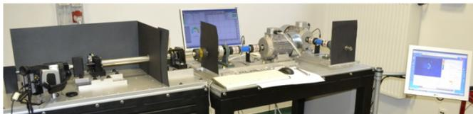
Figure 1: Special purpose equipment for testing non-metallic bearings
