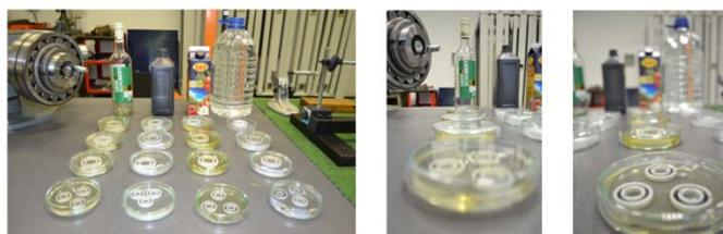
Figure 10: Bearings in different process fluids
