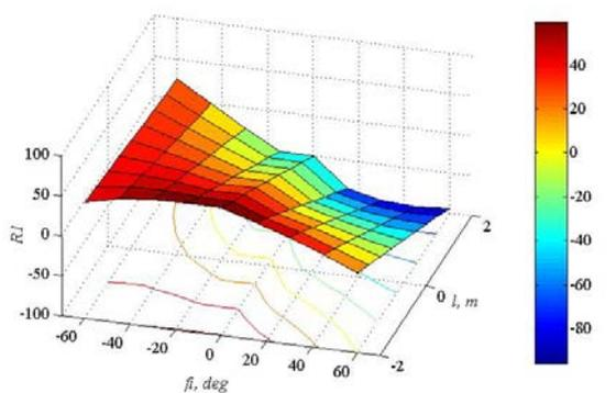
**Fig. 2** The graphic of changing the force in the left hydraulic cylinder depending on the angle of the blade position in the plane and the point of applying unit forces.
