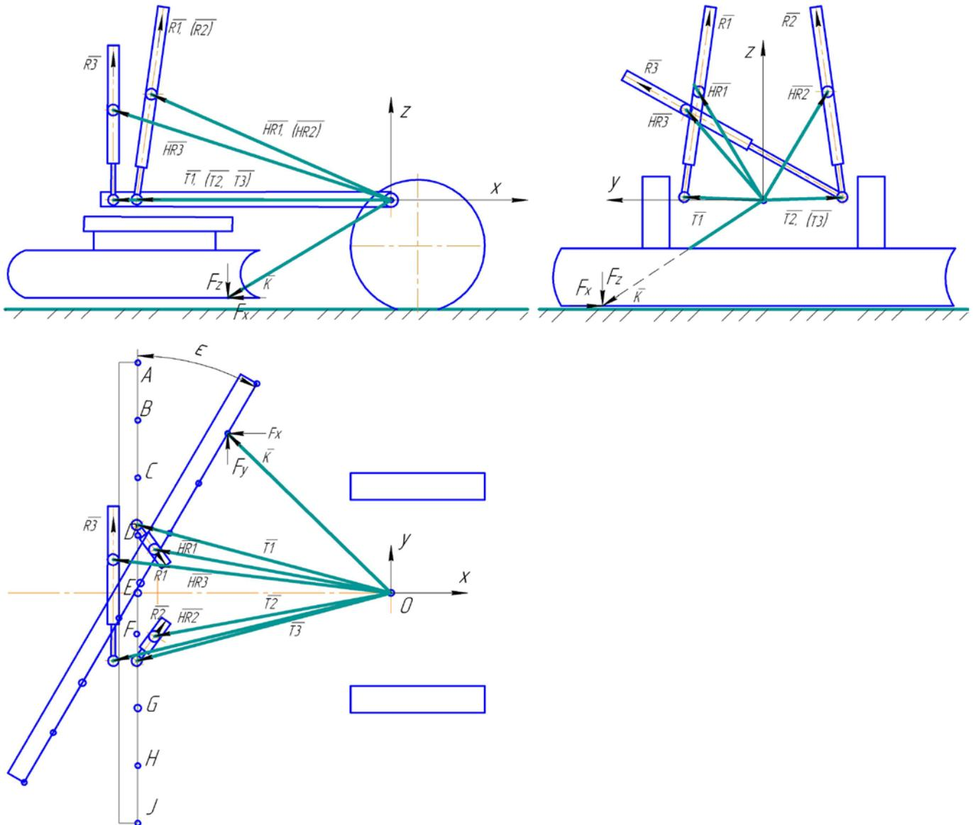
Fig. 1 3-dimensional scheme of applying forces to the motor-grader working attachment
