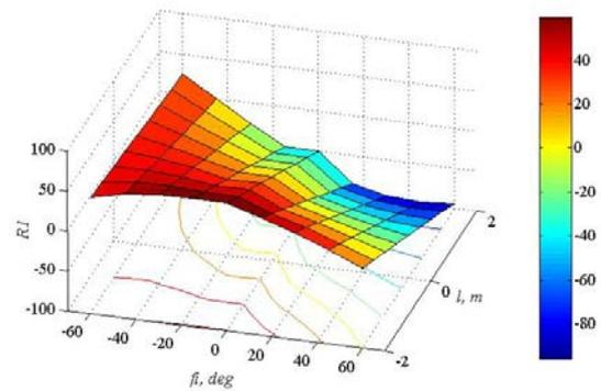
**Fig. 4** The graphic of changing the force in the hydraulic cylinder of the drawbar shift depending on the angle of the blade position in the plane and the point of applying unit forces.
