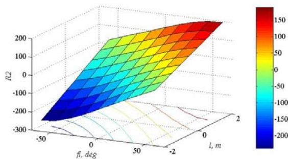
**Fig. 3** The graphic of changing the force in the right hydraulic cylinder depending on the angle of the blade position in the plane and the point of applying unit forces.
