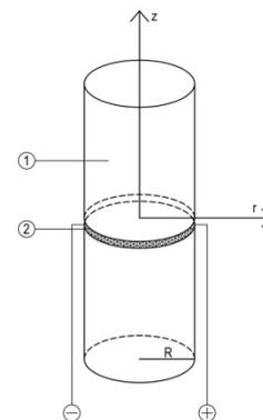
Fig. 1 Setup of experiment 1 – heater, 2 – sample
