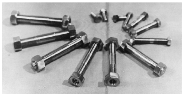
Fig. 1 Bolts used in the automobile and aircraft industries–SPD Ti alloy [4].
