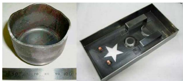
Fig. 2 UFG C-Mn steel sheet forming for automotive industry [5].
