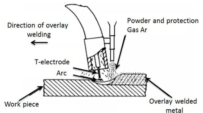
**Fig. 2.** *Welding without melting of powder*
