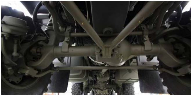
Fig. 3 Front axle of the vehicle T-810 [9].
