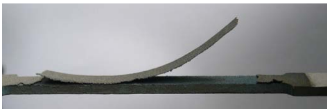
Fig. 5. Delamination of the plasma-sprayed coating with the thickness of 300 μm
