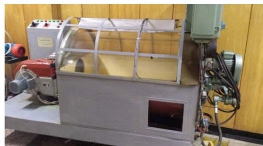
Fig. 2 Testing station for combustion
