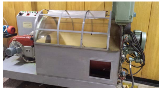
Fig. 2 Testing station for combustion
