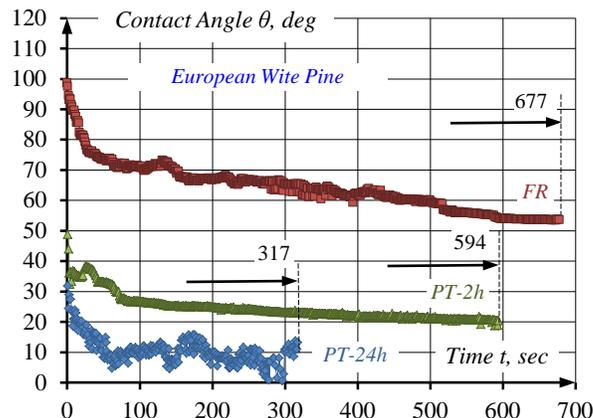
**Fig. 3.** Time-depending change of the contact angle  $\theta$  of basic phosphor and nitrogen containing flame retardant as it advances slowly over the European white pine (*Pinus Sylvestris*) bare (non-plasma treated) sample surface (FR); 2 hours after plasma surface pre-treatment (PT-2h); and 24 hours after plasma surface pre-treatment (PT-24h).
