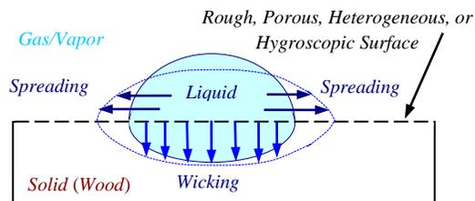
**Fig. 1.** Young-Bikerman-Good model of wetting phenomena - the wetting phenomena on a real surface can be involved by: *i* - spreading of liquid over a solid surface; *ii* - wicking of a liquid into a porous solid such as wood.
