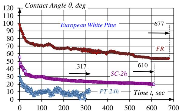
**Fig. 4.** Time-depending change of contact angle  $\theta$  of basic phosphor and nitrogen containing flame retardant as its advance slowly over the European white pine (*Pinus Sylvestris*) bare (non-plasma treated) sample (FR); 2 hours active depolarization after plasma surface pre-treatment (SC-2h); and 24 hours after plasma surface pre-treatment (PT-24h).
