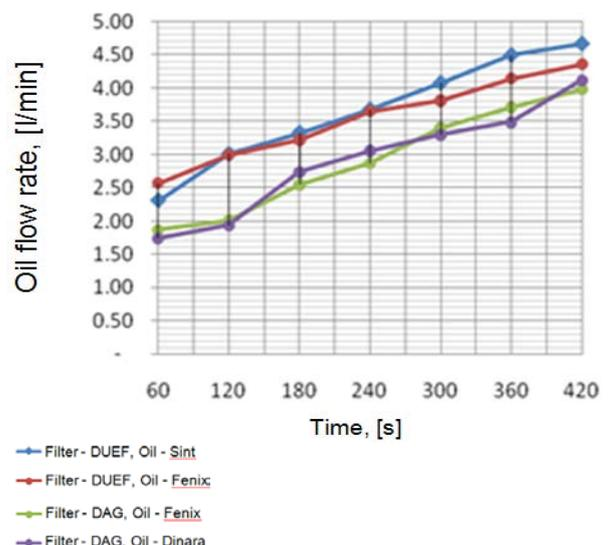
**Fig. 8. Oil flow rate vs time for 2000 rpm**
