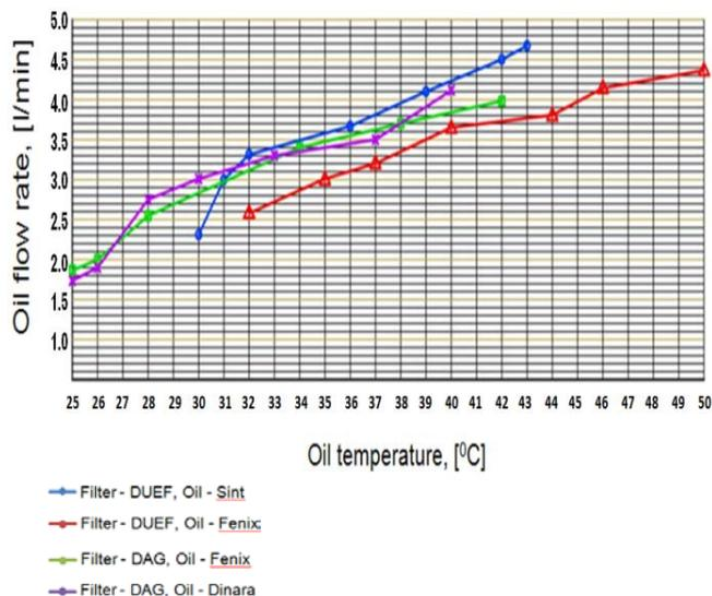
Fig. 10. Oil flow rate vs oil temperature for 2000 rpm
