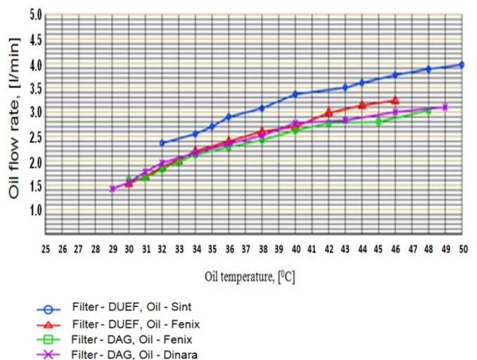
**Fig. 7. Oil flow rate vs oil temperature for 850 rpm**
