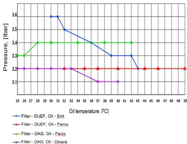
Fig. 9. Oil pressure vs oil temperature for 2000 rpm
