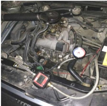
Fig. 1. Performing experiment in Fiat Tipo by installing measuring device
