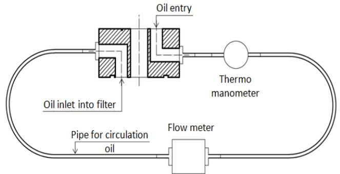
Fig. 3. Connection scheme for measuring performance lubrication system
