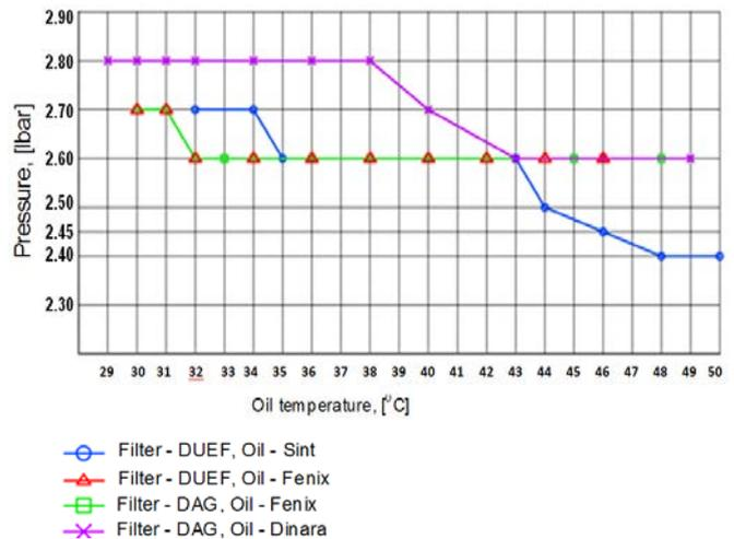
**Fig. 6. Oil pressure vs oil temperature for 850 rpm**
