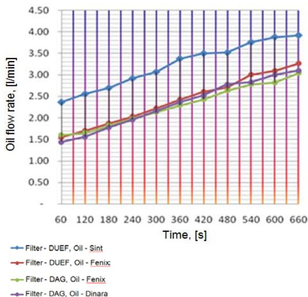
**Fig. 5. Oil flow rate vs time for 850 rpm**
