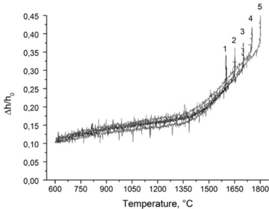
Fig. 2. Linear shrinkage  $\Delta h/h_0$  for  $\beta$ - $\text{Si}_5\text{AlON}_7$  as a function of temperature  $T$  for  $T_{\text{max}} = 1600$  (1),  $1650$  (2),  $1700$  (3),  $1750$  (4), and  $1800^\circ\text{C}$  (5).
