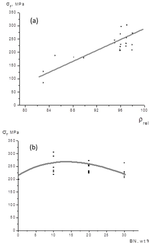
**Fig. 6.** Flexural strength  $\sigma_f$  as a function of: (a) relative density  $\rho_{rel}$  of  $\beta$ -Si<sub>3</sub>AlON<sub>7</sub>-BN ceramics and (b) their BN content ( $\rho_{rel} = 0.95$ – $0.98$ ).
