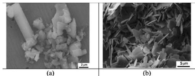
Fig. 1. SEM images of raw  $\beta$ -Si<sub>5</sub>AlON<sub>7</sub> (a) and h-BN (b) powders.
