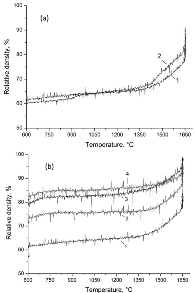
Fig. 4. Relative density  $\rho_{\text{rel}}$  as a function of temperature  $T$  for: (a)  $\beta$ - $\text{Si}_5\text{AlON}_7$  (1) and  $\beta$ - $\text{Si}_5\text{AlON}_7$ - $\text{Y}_2\text{O}_3$  (5 wt %) (2); and (b)  $\beta$ - $\text{Si}_5\text{AlON}_7$  (1),  $\beta$ - $\text{Si}_5\text{AlON}_7$ -BN (10 wt %) (2),  $\beta$ - $\text{Si}_5\text{AlON}_7$ -BN (20 wt %) (3), and  $\beta$ - $\text{Si}_5\text{AlON}_7$ -BN (30 wt %) (4);  $T_{\text{max}} = 1650^\circ\text{C}$ .
