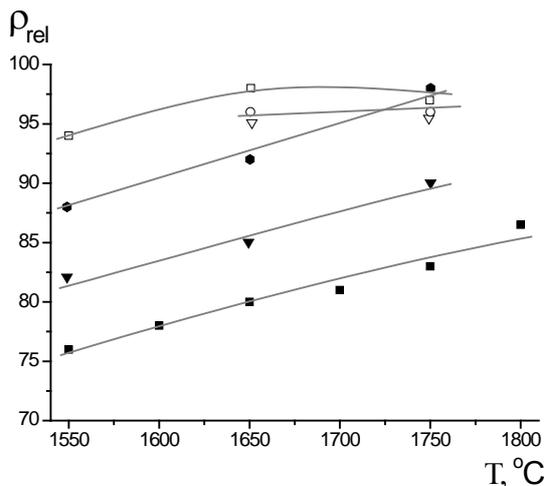
Fig. 3. Relative density  $\rho_{\text{rel}}$  as a function of  $T_{\text{max}}$  for: (■)  $\beta$ - $\text{Si}_5\text{AlON}_7$ , (▼)  $\beta$ - $\text{Si}_5\text{AlON}_7$ - $\text{Y}_2\text{O}_3$  (2.5 wt %), (●)  $\beta$ - $\text{Si}_5\text{AlON}_7$ - $\text{Y}_2\text{O}_3$  (5 wt %), (▽)  $\beta$ - $\text{Si}_5\text{AlON}_7$ -BN (10 wt %), (□)  $\beta$ - $\text{Si}_5\text{AlON}_7$ -BN (20 wt %), (○)  $\beta$ - $\text{Si}_5\text{AlON}_7$ -BN (30 wt %).
