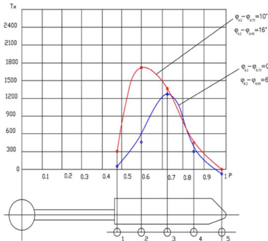
Fig. 6. Diagram of dependence of the VGR thrust from the blades twist change for the maximal diameter  $D_{max}$  of the rotor, rotational speed  $n = 200$  RPM and setting angle  $\varphi = 5^0$ .
