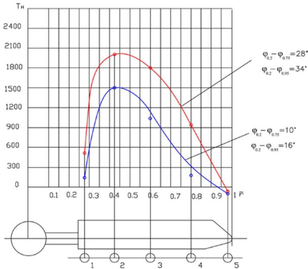
Fig. 5. Diagram of dependence of the VGR thrust from the blades twist change for the minimal diameter  $D_{min}$  of the rotor, rotational speed  $n = 300$  RPM and setting angle  $\varphi = 5^0$ .
