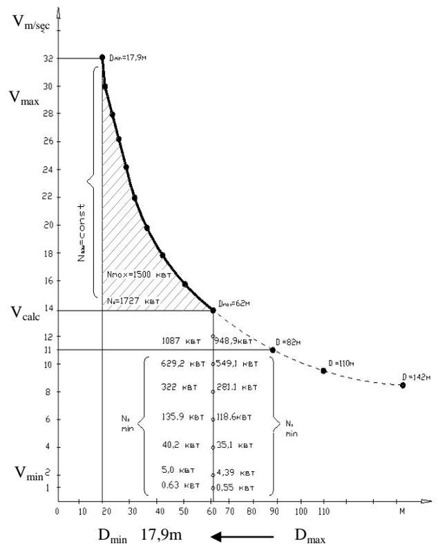
Fig. 9. Necessary combination of the rotor diameter and wind speed for acquisition of the planned power of wind station.
