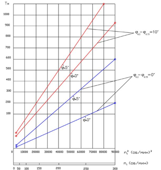
Fig. 8. Diagram of dependence of the VGR thrust from the rotor rotational speed for the maximal diameter  $D_{max}$ .
