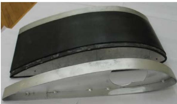
Fig. 3. Stand for static tests and blade with flexible elements and rib.
