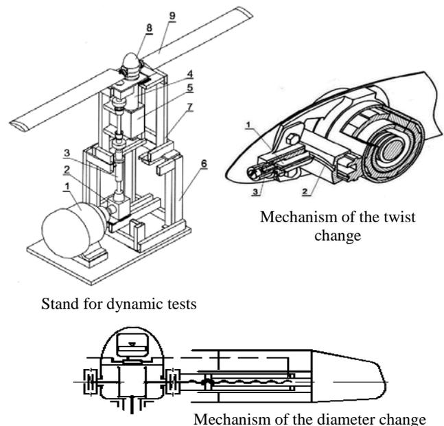
Fig. 1. Mechanisms for management of parameters of the VGR and stand for their tests.
