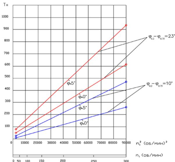
Fig. 7. Diagram of dependence of the VGR thrust from the rotor rotational speed for the minimal diameter  $D_{min}$ .
