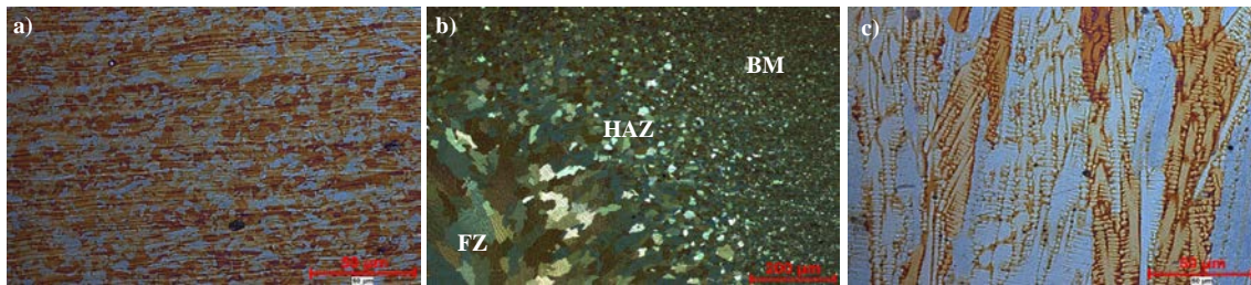
Fig.2 Microstructural changes from the BM to the FZ via optical microscopy observations. (a) BM, (b) transition zone between FZ and BM, (c) FZ. (The joint with welding time of 300 ms).
