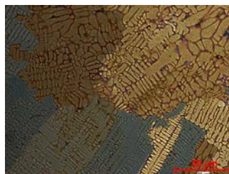
Fig.3 Interdendritic micro-pores in FZ. (The joint with welding time of 300 ms).
