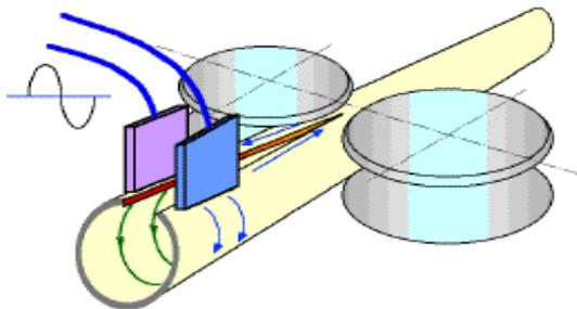
Fig.1 Schematic illustration of HFERW
