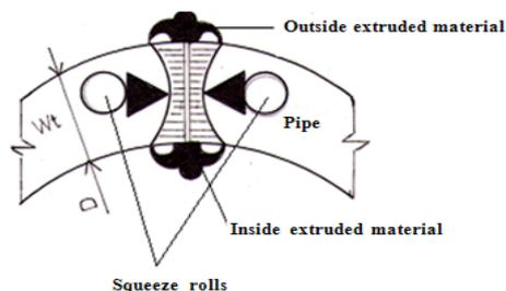
Fig.2 High frequency forge type weld
