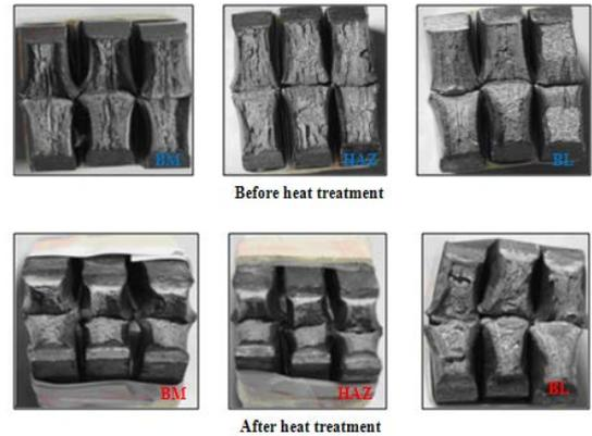
Fig.10 Fracture surfaces from Charpy-V-notch (CVN) testing
