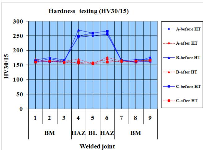
Fig.9 Hardness (HV30/15) testing results
