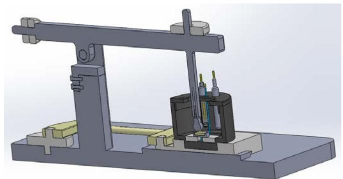
**Fig. 1** Schematic representation of reciprocating tribometer coupled with electrochemical cell.
