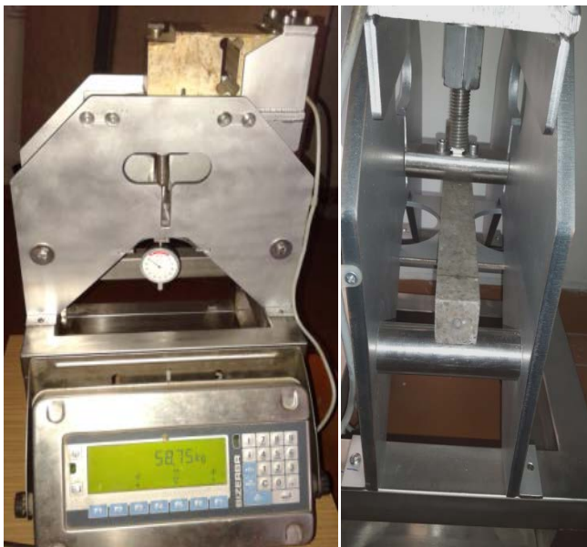
Fig.6. Experimental setting for determining the static modulus
