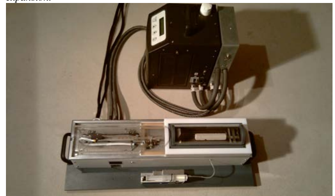
Fig. 1 Dilatometer for measurement of moisture and temperature induced expansion.
