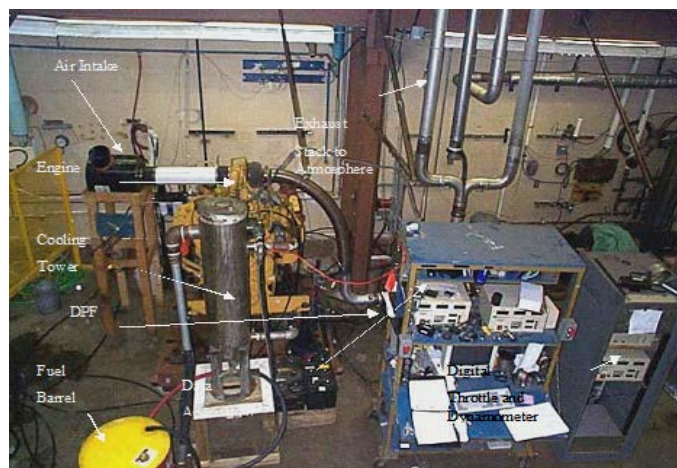
Fig. 4 Engine setup with, instrumentation rack, and dynamometer controllers
