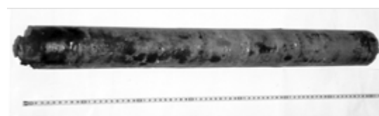
Fig. 2 Zirconium ingot obtained by EBMR of zirconium sponge.
