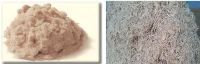
Fig 2: Fine fibers use of the surface layer(left), coarse fibers use of core layers (right)
