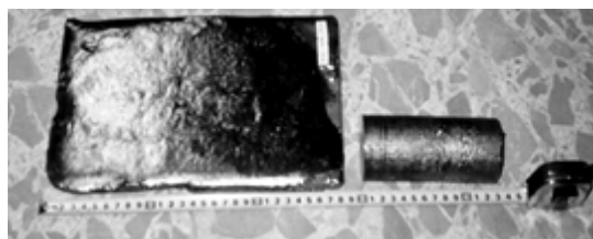
Fig. 4 Titanium targets regenerated by EBMR.
