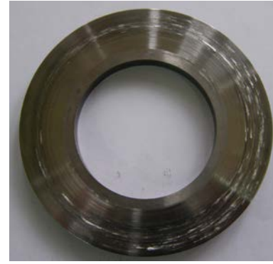
Fig. 5 The photograph of the G51320 steel counterface worn surface. The applied load is 10 N, and the sliding velocity is 4 m/s.
