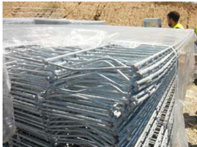
Figure 6 Mechanically damaged panels
