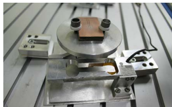
Fig. 2. The device for measurement of torque.
